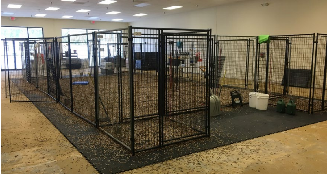
Figure 1. Airlock entrances to the yard with two gates, one into the airlock and one into the yard, to prevent dogs from escaping and to give the handler a safe space to remove the dog's leash or other equipment before entering the yard.
